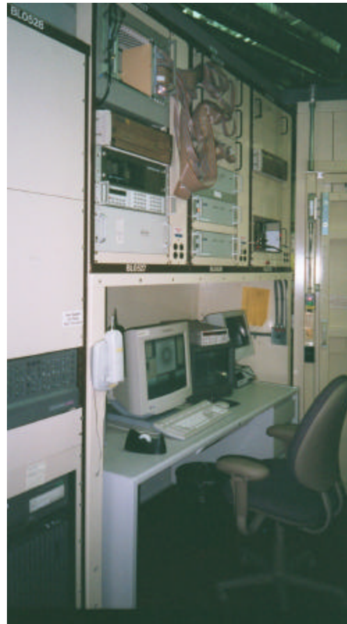
Data collection system at the ALS Beamline 5. Goniostat and beamline optics are in the hutch to the right of the chair.
